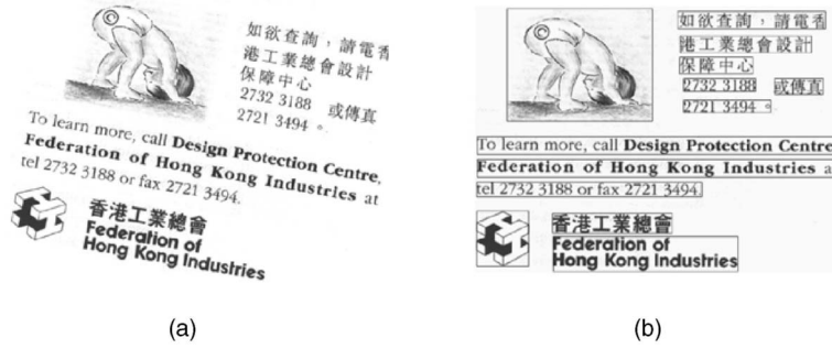
Fig. 2. Component Block Representation (CBR) of a document image. (a) The scanned grayscale image. (b) The CBR of (a) (component blocks are drawn as the rectangular bounding boxes of the corresponding document image regions).
